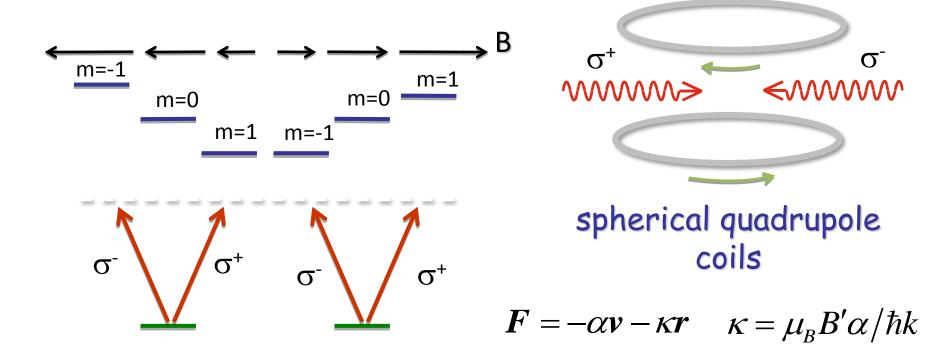
Load the MOT from a slowed beam, or using the low velocity thermal tails of vapor cell. It is a dissipative trap that dramatically increases the phase space density. Can collect up to ~10<sup>10</sup> atoms.
