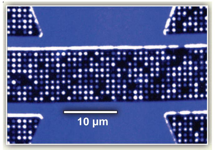
Chip scale nano fabrication of single spin arrays in diamond. D. M. Toyli et al., Nano Lett. 10, 3168 (2010).
