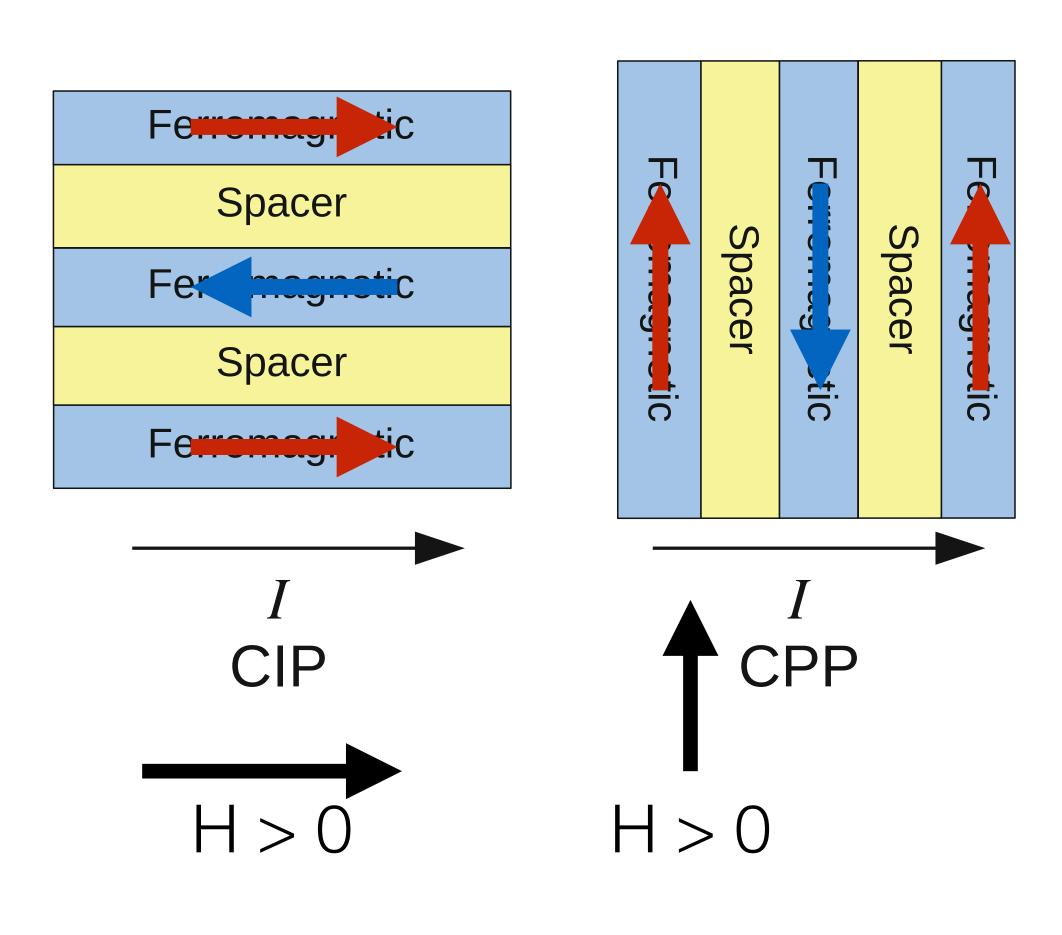
Two geometries for GMR: Current-in-plane (CIP) Current-perpendicular-to-plane (CPP)
