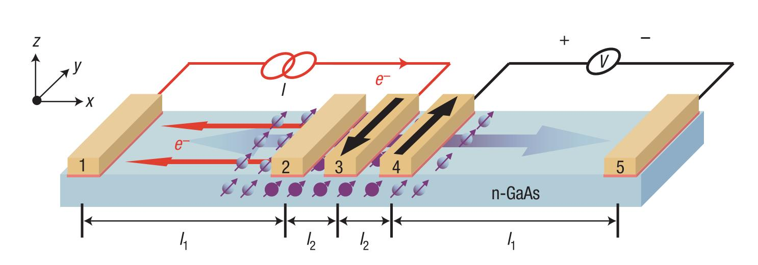
Ferromagnetic contacts can source spin polarized current in a semiconductor and detect it via a 'spin valve' effect.
