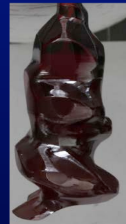
\text{Sm}_2\text{Ti}_2\text{O}_7 grown by Czochralski (IKZ, Berlin)
